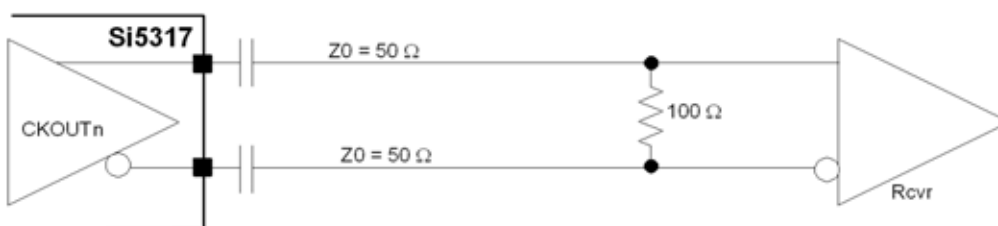
Figure 11. Typical Differential Output Circuit
