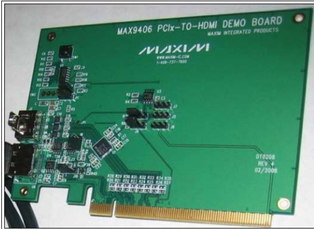
Figure 8. A MAX9406-based HDMI/DVI level-shifter plug-in card.
