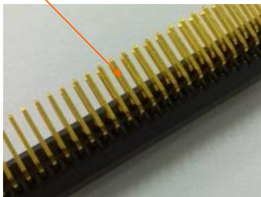
Yellow color at solder tail area
