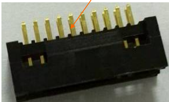
Yellow color at solder tail area
