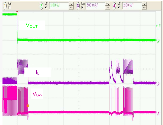
Figure 16. Metallic Short Applied at V OUT , 50μs/div.
