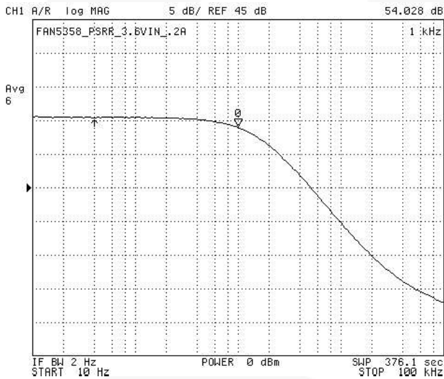
Figure 19. Power Supply Rejection Ratio at 200mA Load
