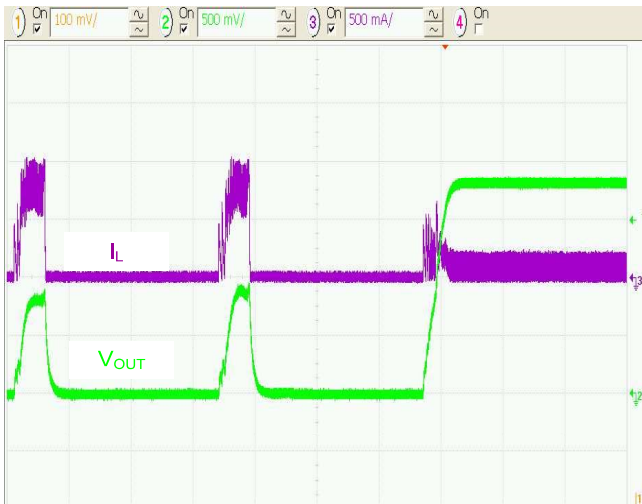
Figure 17. Overload Recovery to Light Load, 100µs/div.
