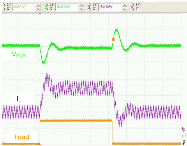
Figure 15. Load Transient 200 to 500mA, 3.6V IN , 5μs/div.
