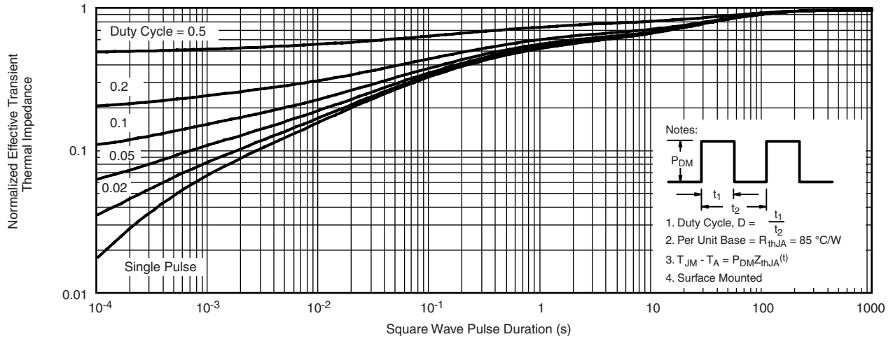
Normalized Thermal Transient Impedance, Junction-to-Ambient
