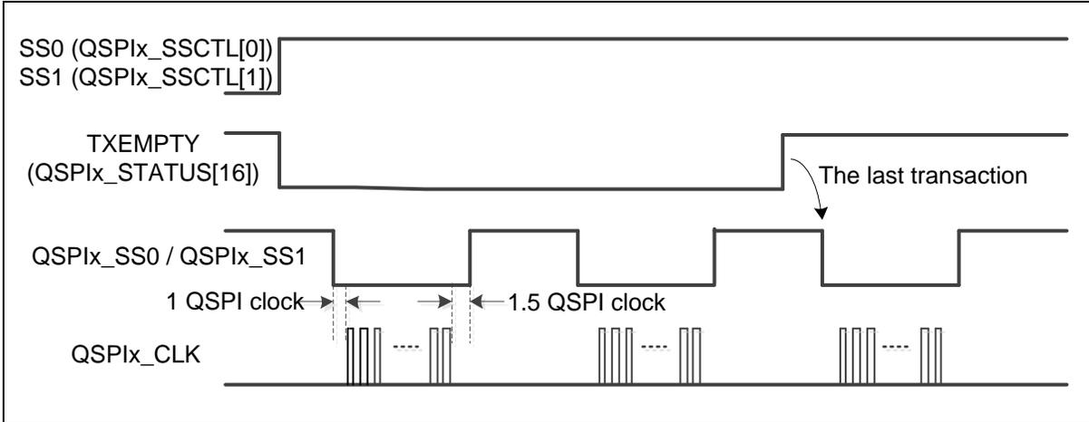
Figure 6.18-6 Automatic Slave Selection (SSACTPOL = 0, SUSPITV > 0x2)
