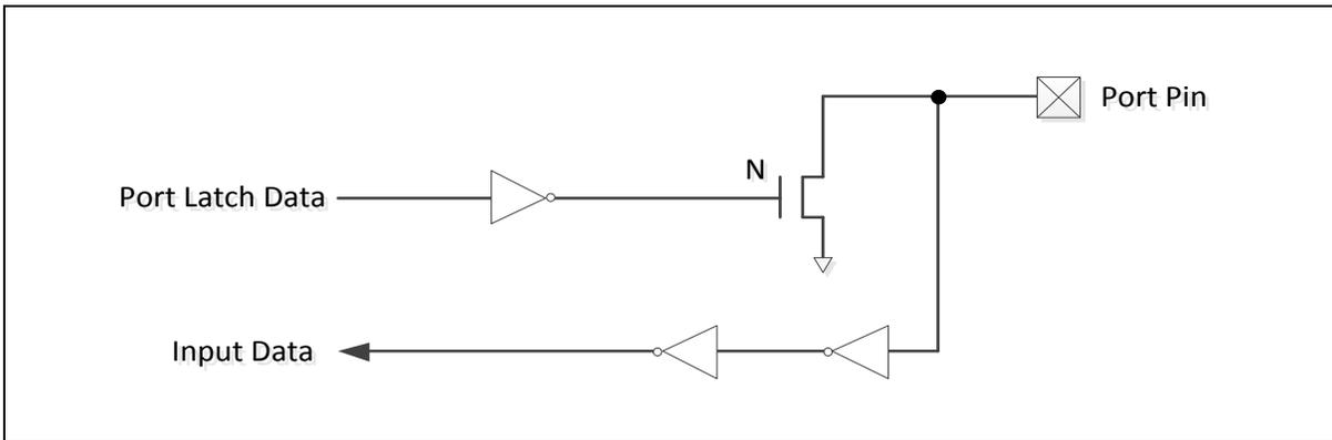
Figure 6.7-3 Open-Drain Output
