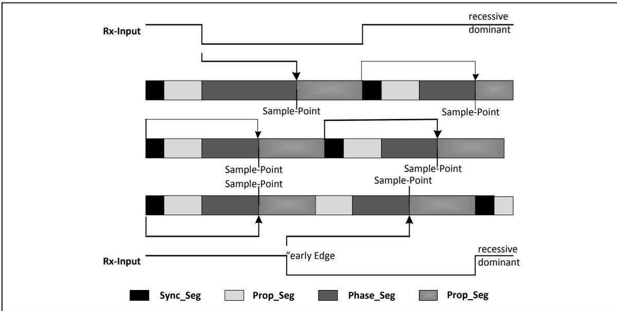
Figure 6.23-9 Synchronization on “Late” and “Early” Edges
