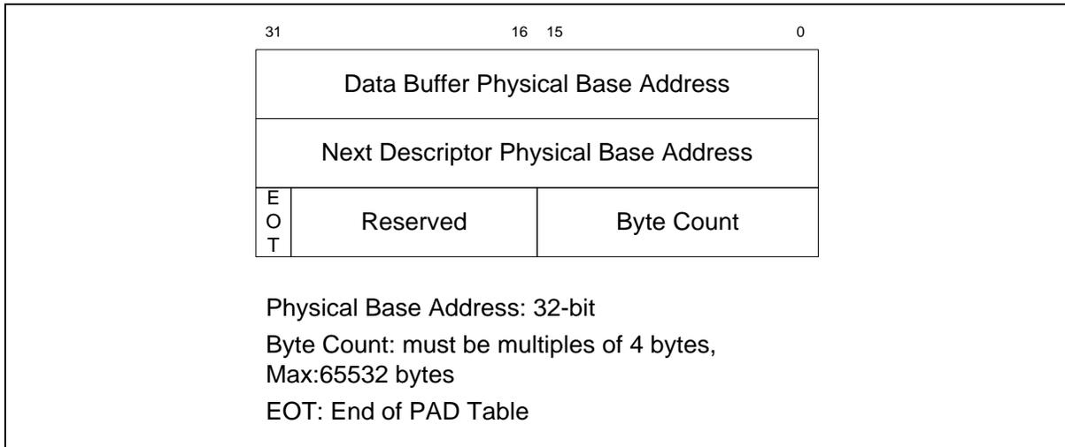
Figure 6.25-2 PAD (Physical Address Descriptor) Table Format
