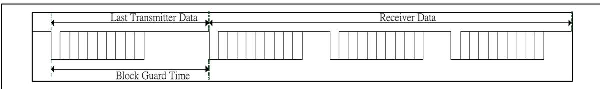
Figure 6.15-11 Receive Direction Block Guard Time Operation
