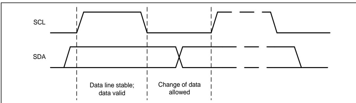
Figure 6.16-5 Bit Transfer on the I<sup>2</sup>C Bus
