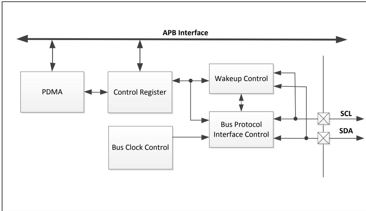
Figure 6.16-1 I<sup>2</sup>C Controller Block Diagram
