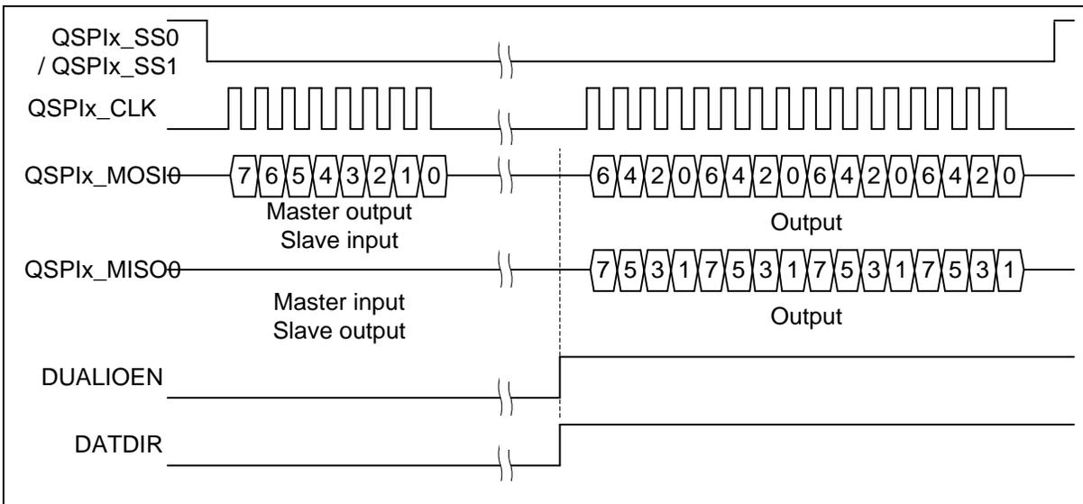
Figure 6.18-14 Bit Sequence of Dual Output Mode
