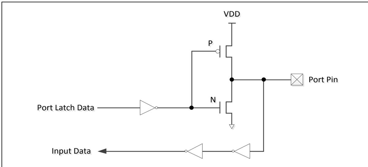
Figure 6.7-2 Push-Pull Output
