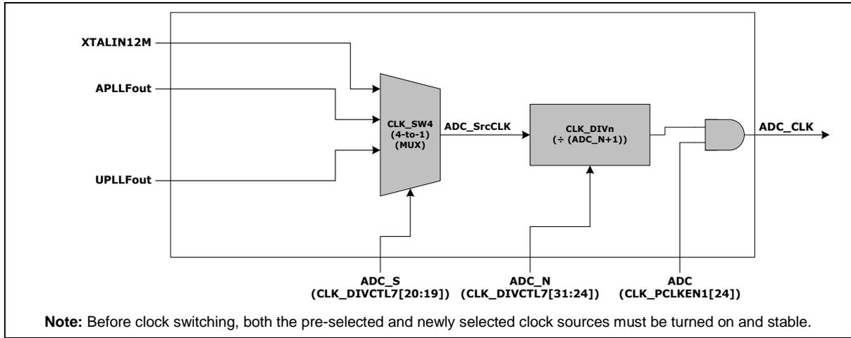
Figure 6.3-2 ADC Controller Clock Divider Block Diagram
