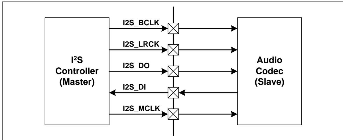
Figure 6.19-2 I<sup>2</sup>S Interface Signal of Master Mode
