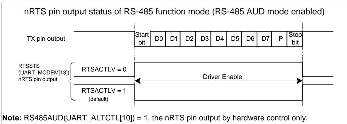
Figure 6.14-25 RS-485 nRTS Driving Level in Auto Direction Mode
