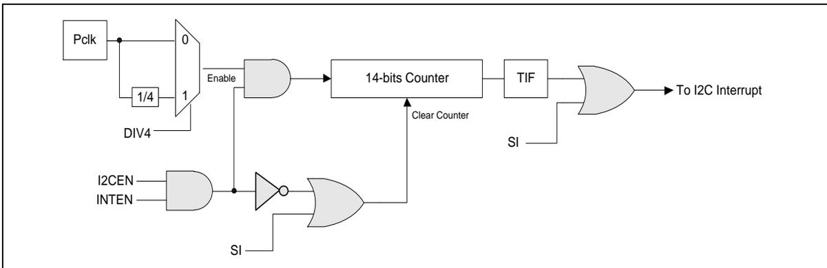
Figure 6.16-20 I<sup>2</sup>C Time-out Count Block Diagram
