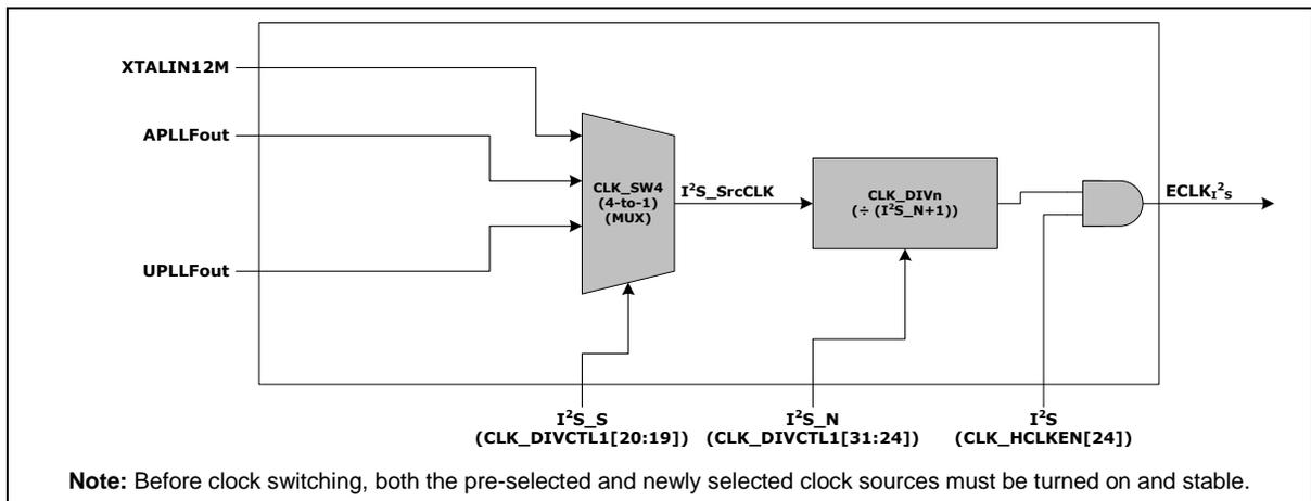
Figure 6.3-6 I<sup>2</sup>S Controller Clock Divider Block Diagram
