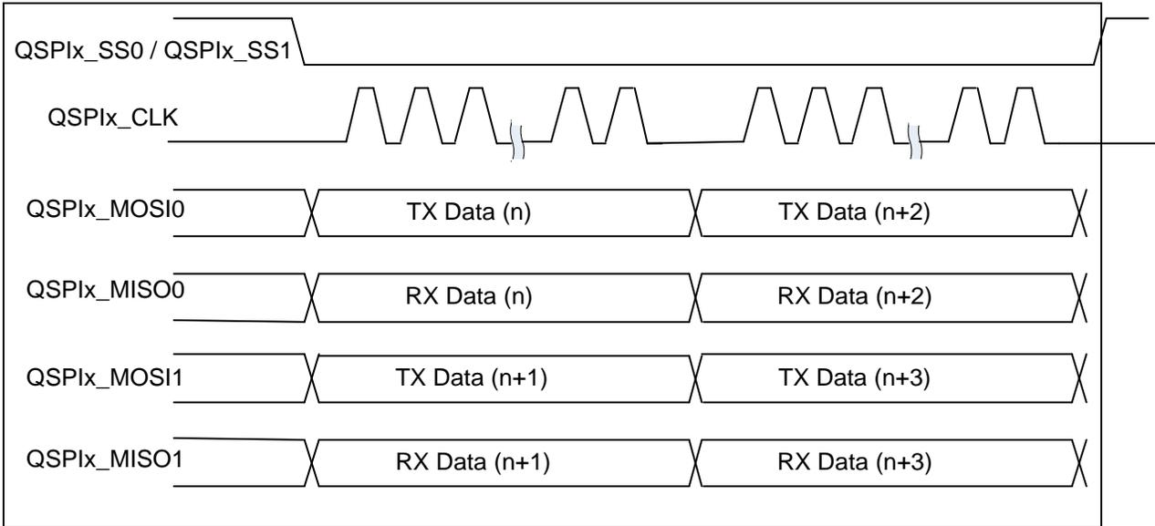
Figure 6.18-13 Two-bit Transfer Mode Timing (Master Mode)
