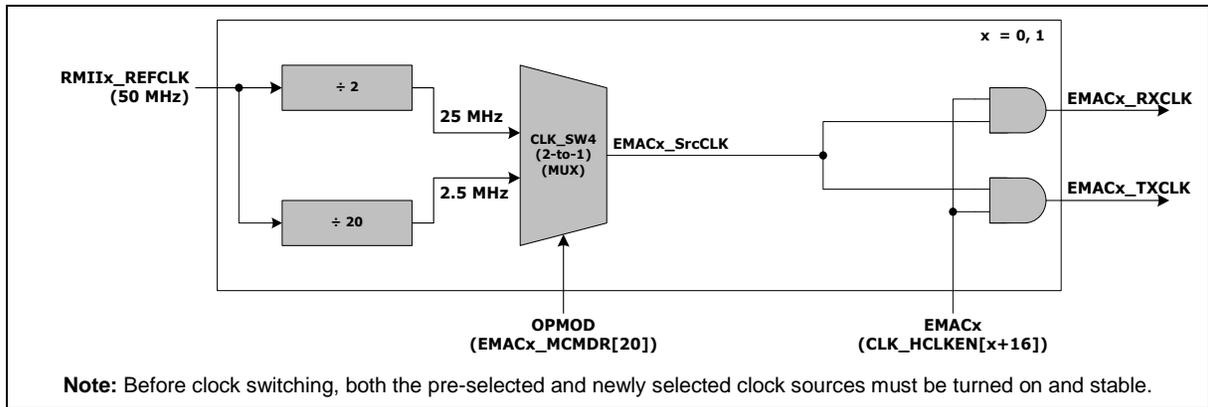
Figure 6.3-5 Ethernet MAC Controller Clock Divider Block Diagram
