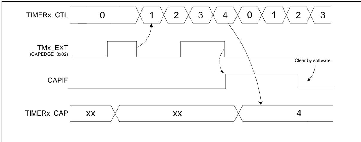
Figure 6.9-6 External CaptureTrigger-Counting Mode (CAPCNTMD (TIMERx\_CTL[20] is 1))
