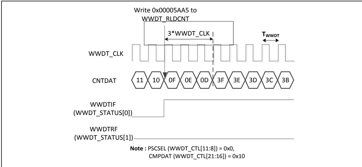
Figure 6.12-5 WWDT Reload Counter When CNTDAT < CMPDAT
