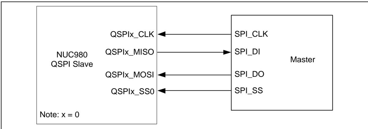
Figure 6.18-4 QSPI Full-Duplex Slave Mode Application Block Diagram
