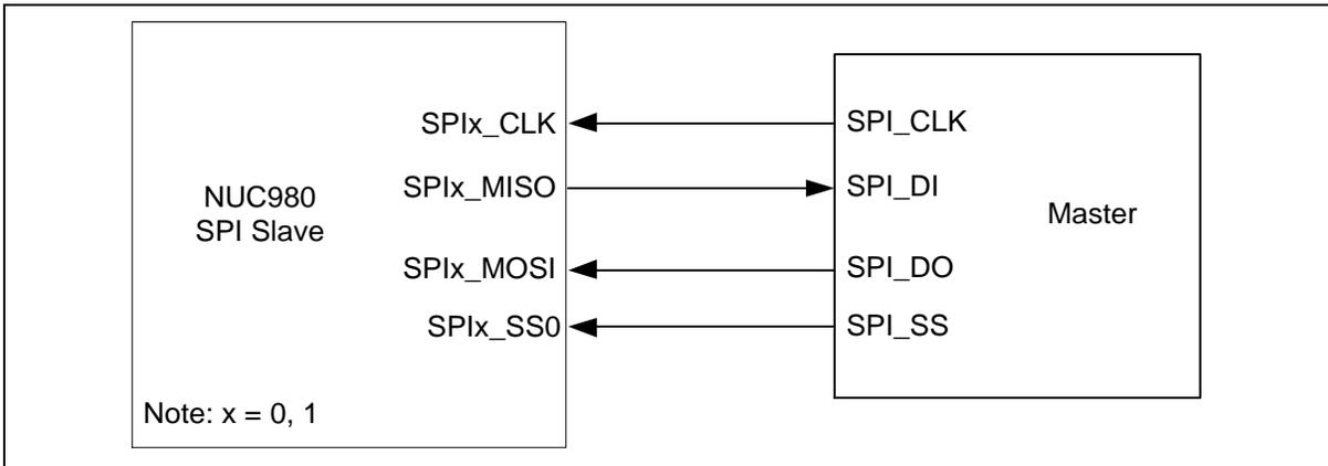
Figure 6.17-4 SPI Full-Duplex Slave Mode Application Block Diagram
