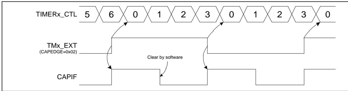
Figure 6.9-7 External Capture/Reset Counter Mode (CAPCNTMD (TIMERx\_CTL[20] is 0))
