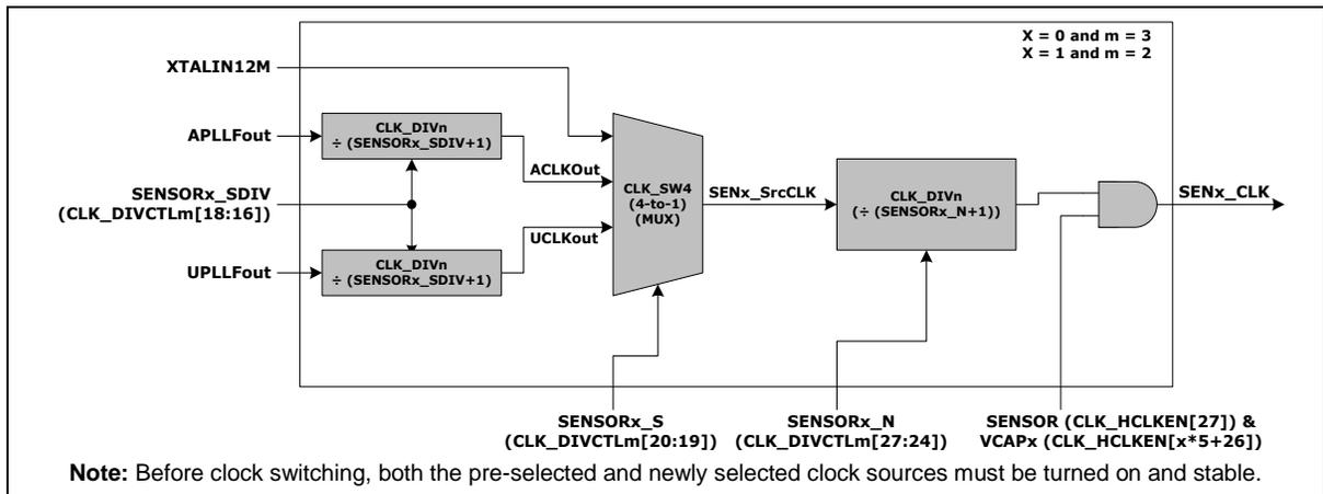
Figure 6.3-9 CMOS Sensor Controller Divider Block Diagram
