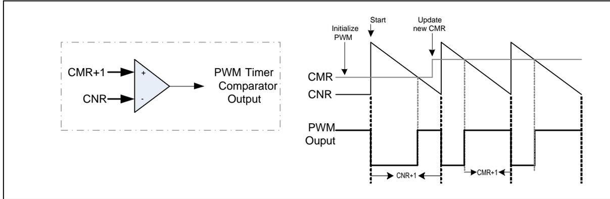
Figure 6.10-2 Legend of Internal Comparator Output of PWM-Timer
