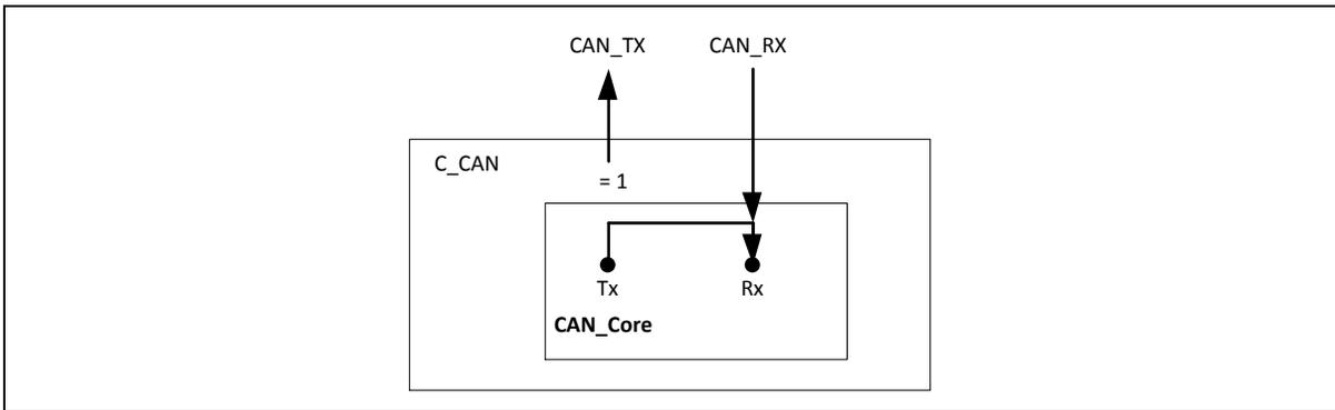
Figure 6.23-2 CAN Core in Silent Mode
