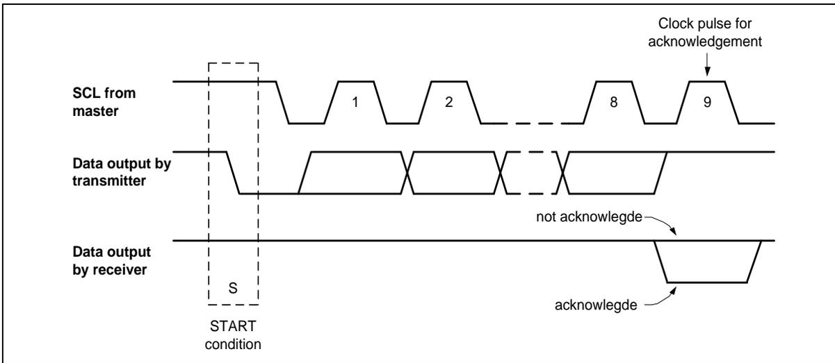
Figure 6.16-6 Acknowledge on the I<sup>2</sup>C Bus
