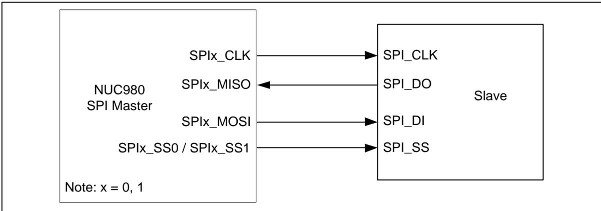
Figure 6.17-3 SPI Full-Duplex Master Mode Application Block Diagram
