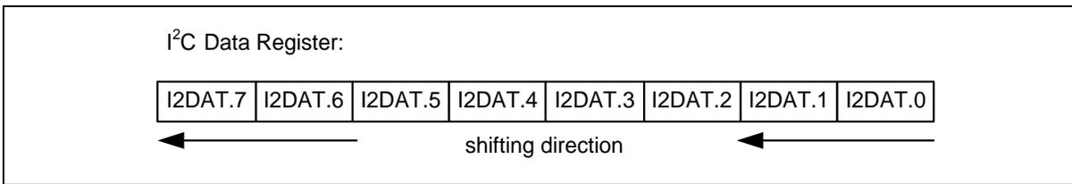
Figure 6.16-19 I<sup>2</sup>C Data Shifting Direction
