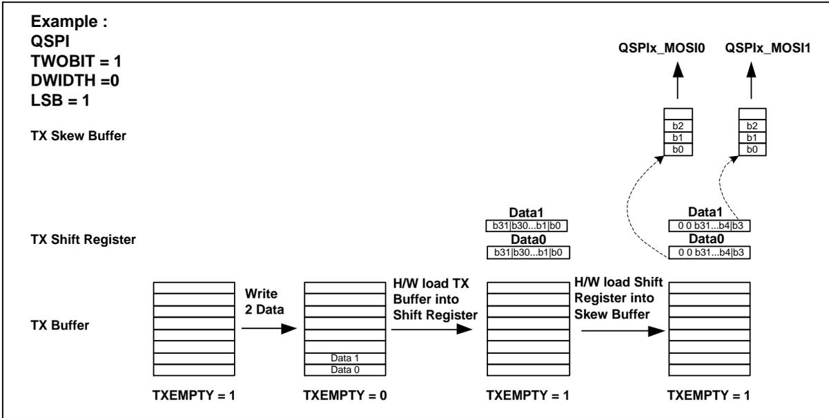
Figure 6.18-22 Two-bit Transfer Mode FIFO Buffer Example
