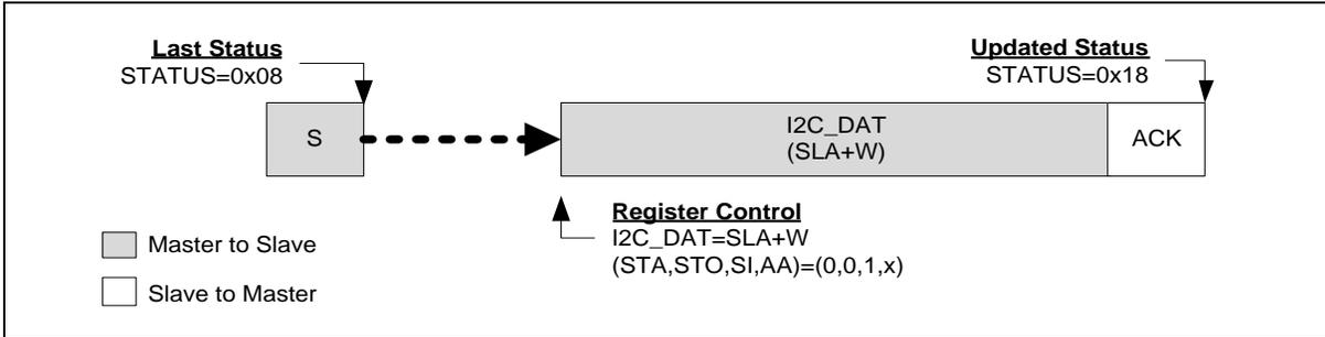
Figure 6.16-11 Control I<sup>2</sup>C Bus according to the Current I<sup>2</sup>C Status
