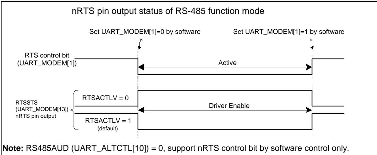
Figure 6.14-26 RS-485 nRTS Driving Level with Software Control
