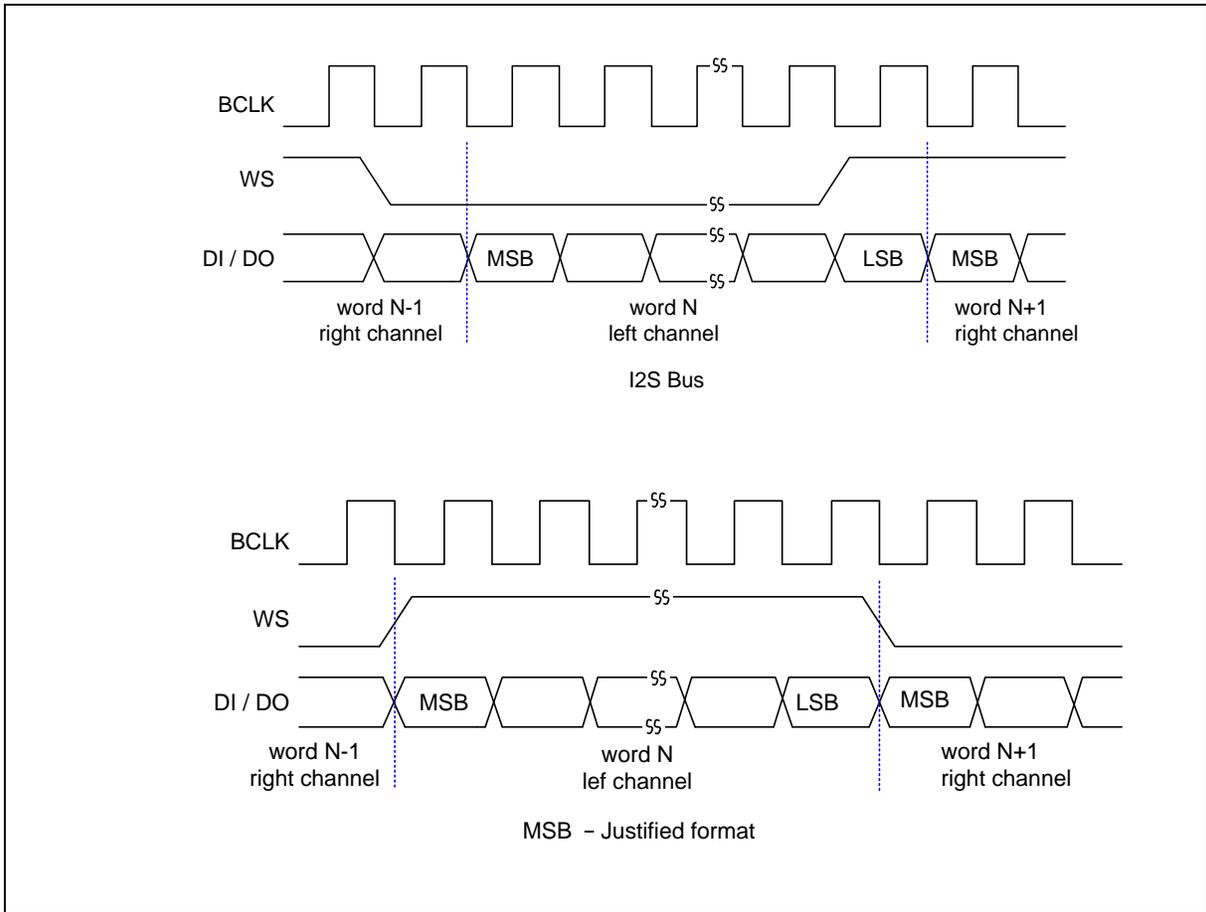
Figure 6.19-4 I<sup>2</sup>S MSB-Justified Format
