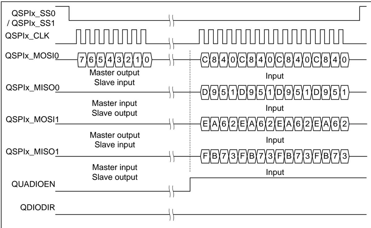
Figure 6.18-17 Bit Sequence of Quad Input Mode
