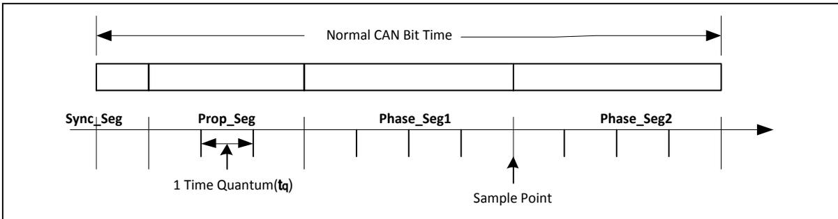
Figure 6.23-7 Bit Timing
