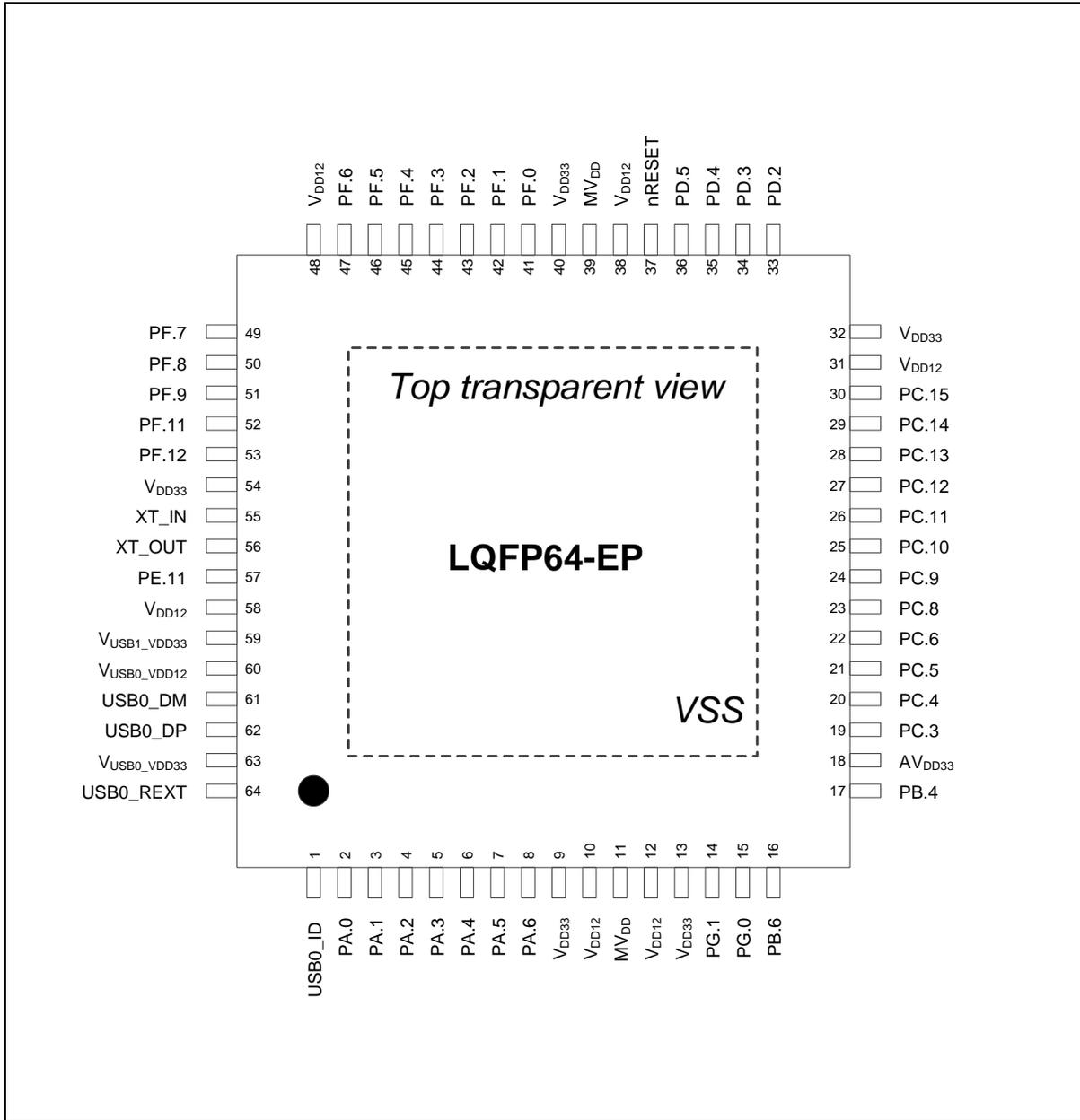
Figure 4.1-1 NUC980DRxxY LQFP 64-pin with EX-PAD Diagram
