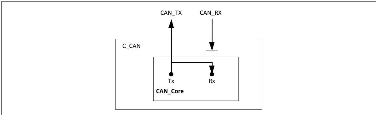
Figure 6.23-3 CAN Core in Loop Back Mode
