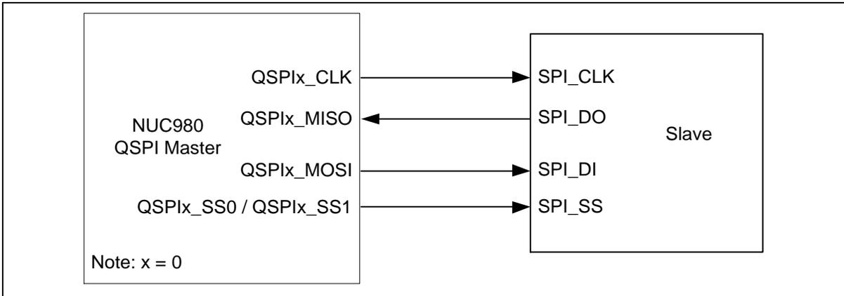
Figure 6.18-3 QSPI Full-Duplex Master Mode Application Block Diagram
