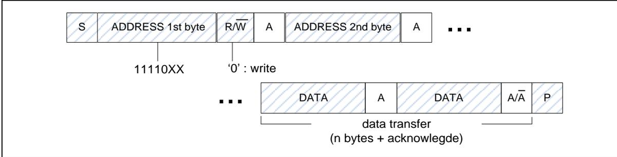
Figure 6.16-9 Master Transmits Data to Slave by 10-bit
