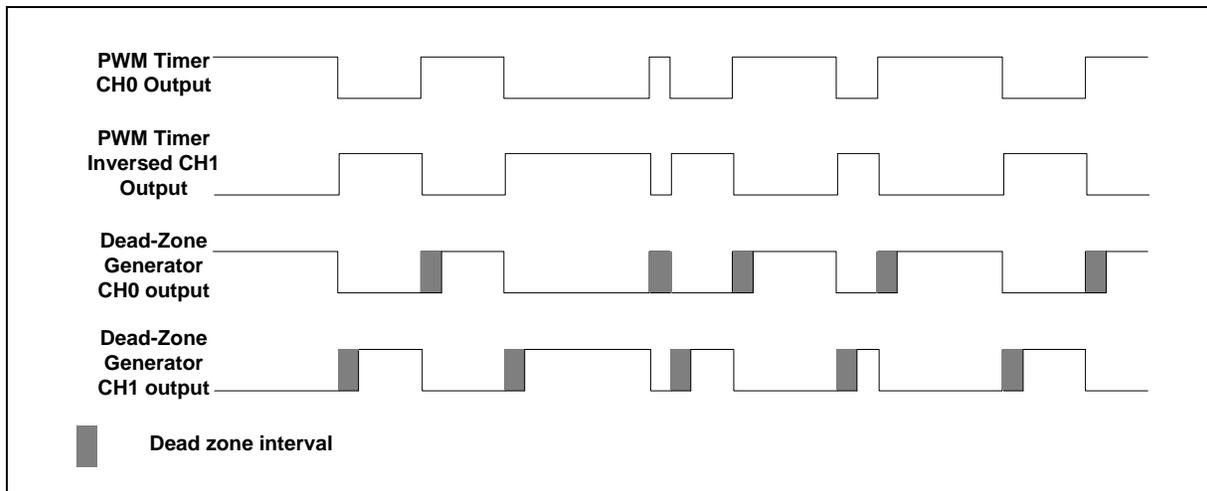
Figure 6.10-5 Paired PWM Output with Dead-Zone Generation Operation
