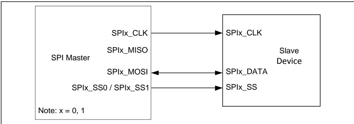
Figure 6.17-10 SPI Half-Duplex Master Mode Application Block Diagram
