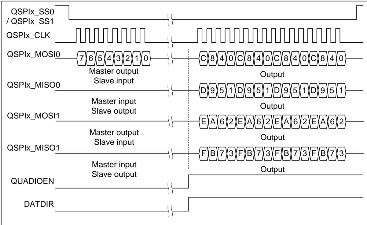
Figure 6.18-16 Bit Sequence of Quad Output Mode
