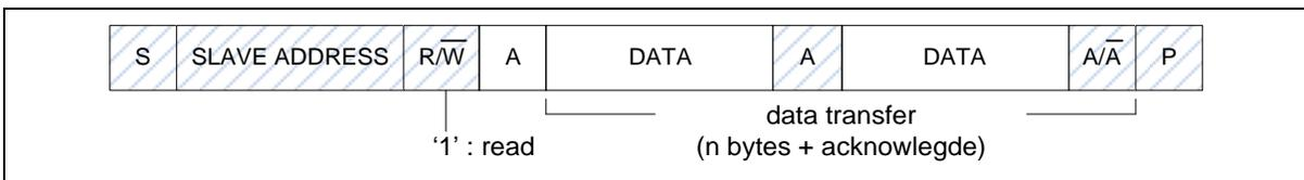
Figure 6.16-8 Master Reads Data from Slave by 7-bit
