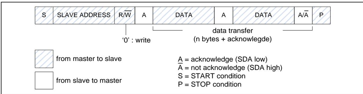
Figure 6.16-7 Master Transmits Data to Slave by 7-bit
