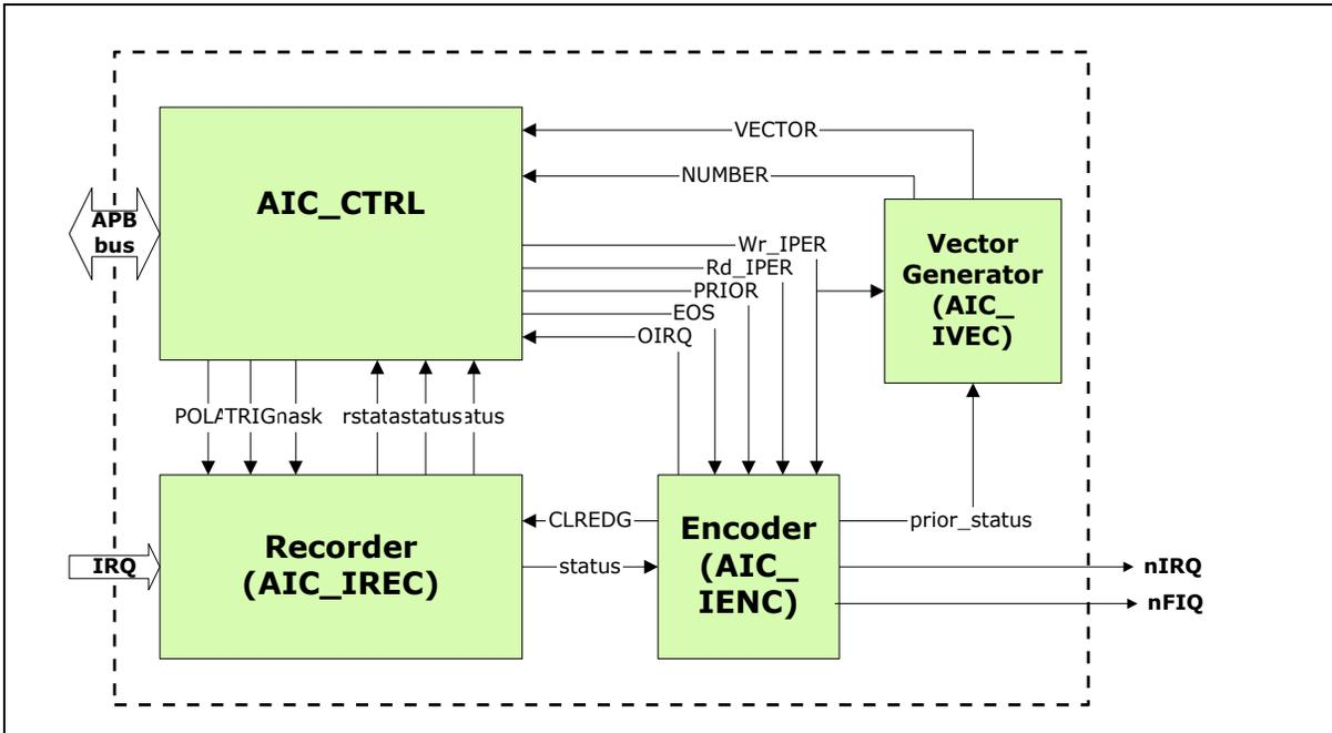
Figure 6.4-1 Advanced Interrupt Controller (AIC) Block Diagram
