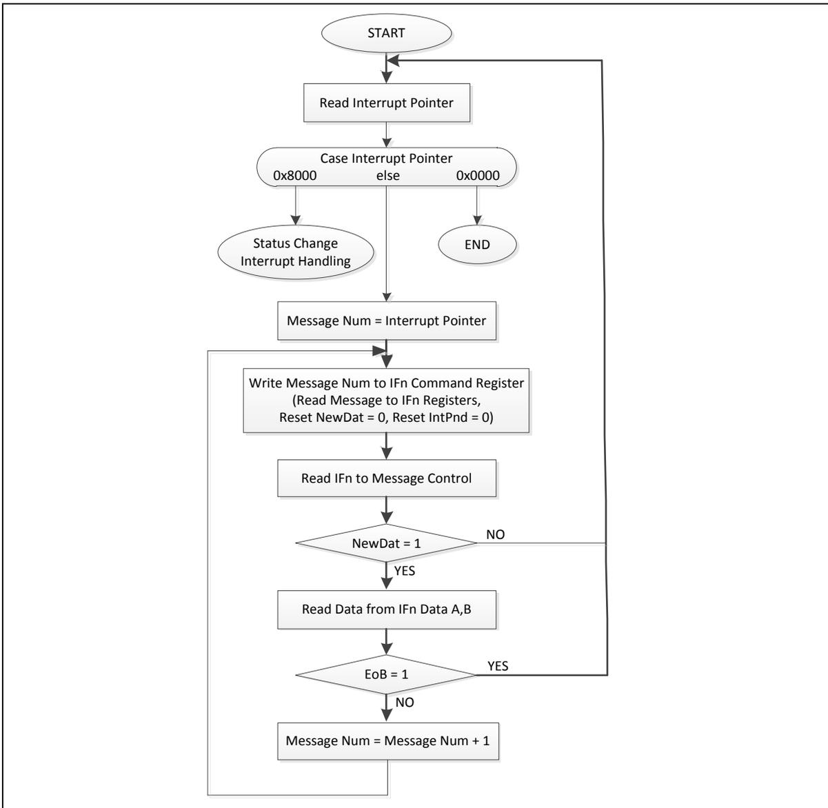
Figure 6.23-6 Application Software Handling of a FIFO Buffer
