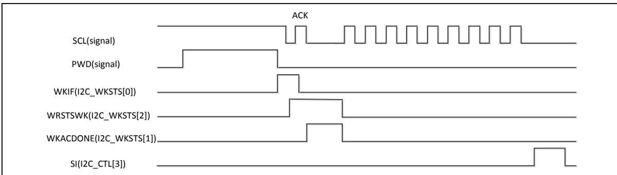
Figure 6.16-21 I<sup>2</sup>C Wake-Up Related Signals Waveform
