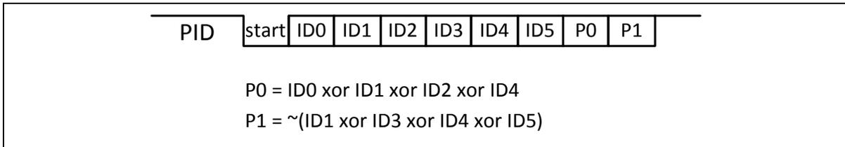
Figure 6.14-21 LIN Frame ID and Parity Format
