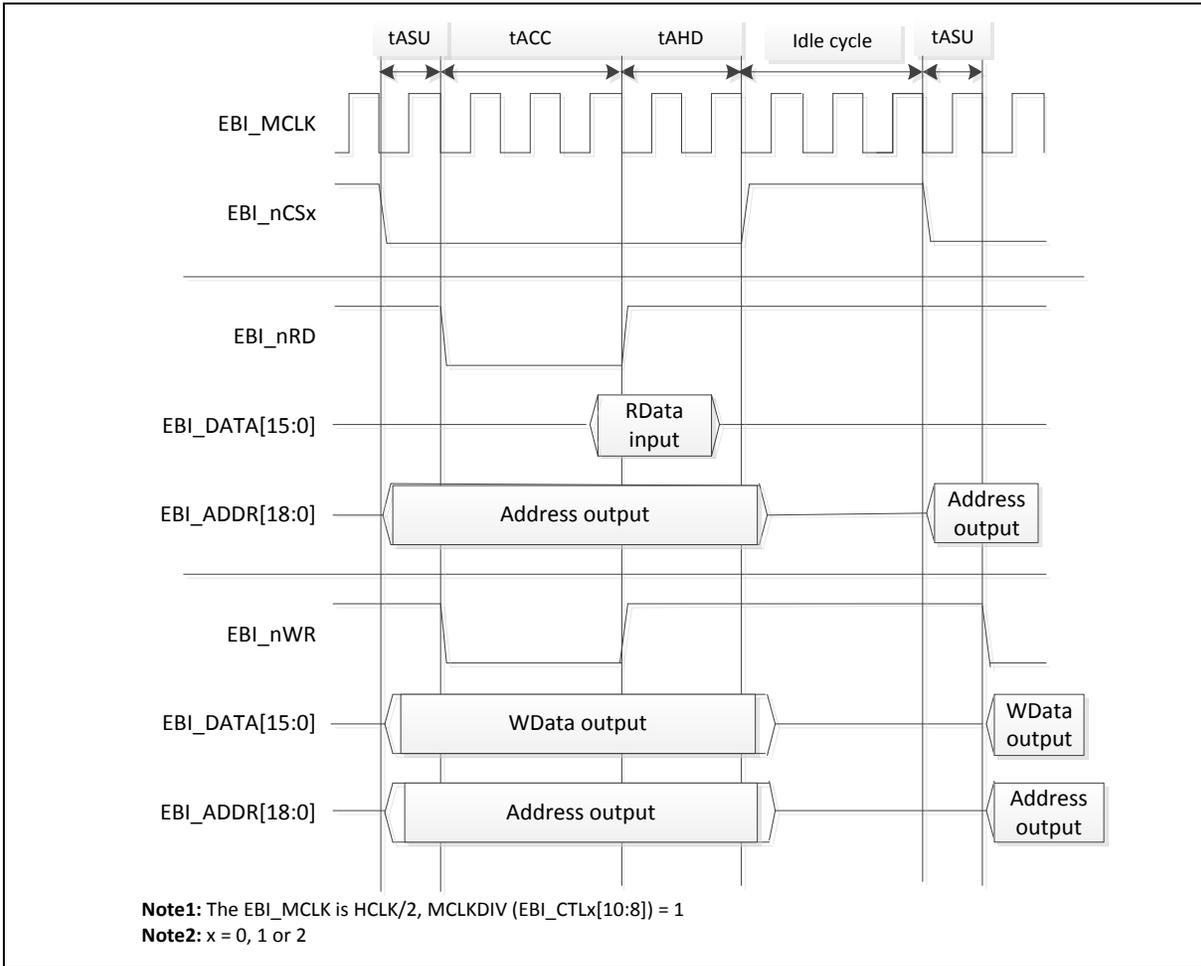
Figure 6.6-5 Timing Control Waveform for Insert Idle Cycle
