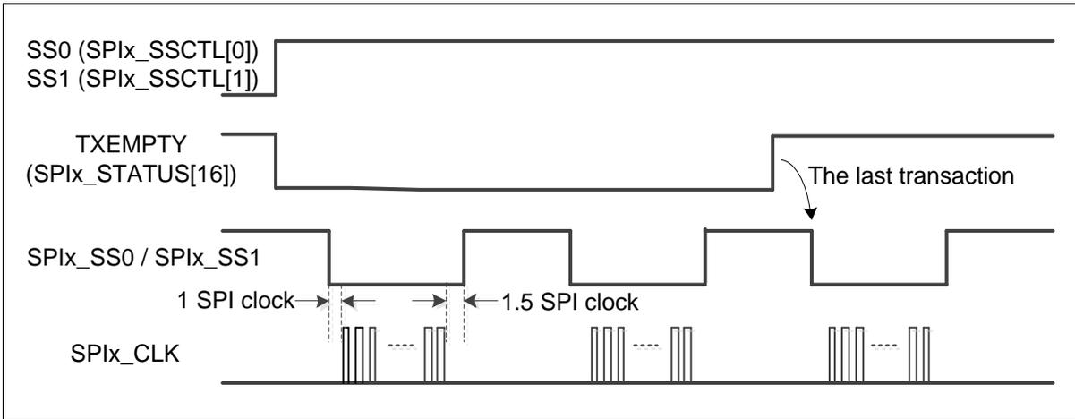
Figure 6.17-6 Automatic Slave Selection (SSACTPOL = 0, SUSPITV > 0x2)
