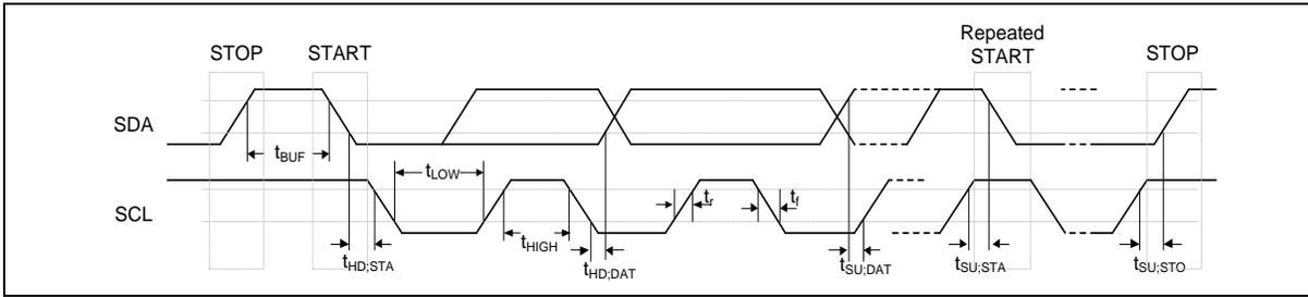
Figure 6.16-2 I<sup>2</sup>C Bus Timing
