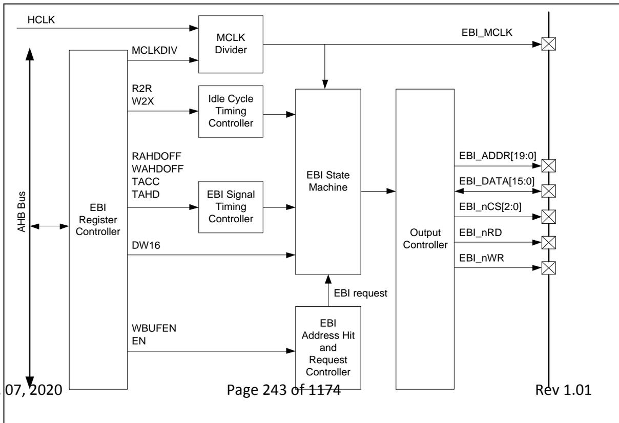
Figure 6.6-1 EBI Block Diagram
