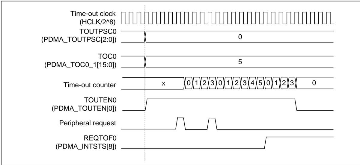
Figure 6.8-6 Example of PDMA Channel 0 Time-out Counter Operation
