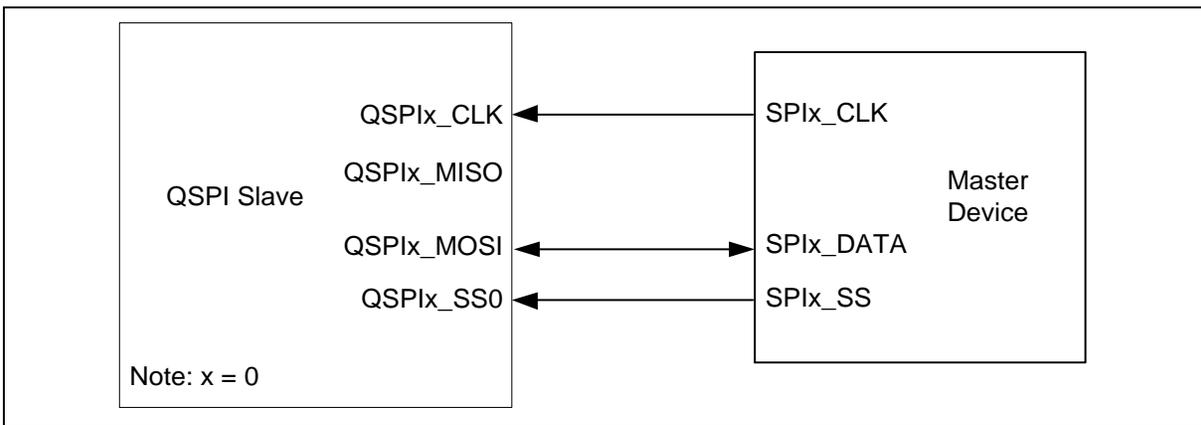
Figure 6.18-11 QSPI Half-Duplex Slave Mode Application Block Diagram
