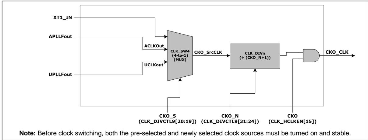
Figure 6.3-7 Reference Clock Output Divider Block Diagram
