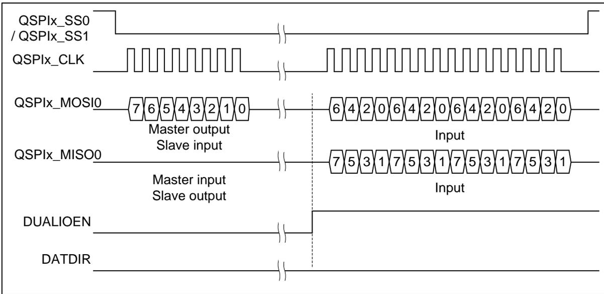
Figure 6.18-15 Bit Sequence of Dual Input Mode
