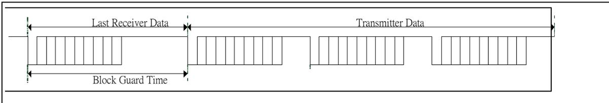
Figure 6.15-10 Transmit Direction Block Guard Time Operation
