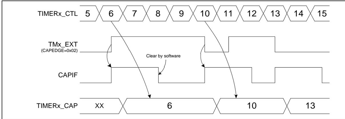
Figure 6.9-5 External CaptureFree-Counting Mode (CAPCNTMD (TIMERx\_CTL[20] is 0))
