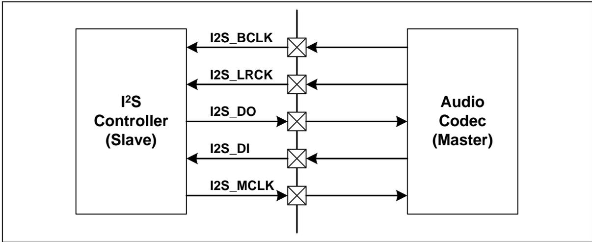
Figure 6.19-3 I<sup>2</sup>S Interface Signal of Slave Mode
