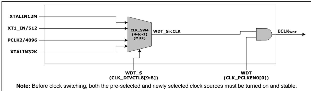
Figure 6.3-12 Watchdog Timer Clock Divider Block Diagram
