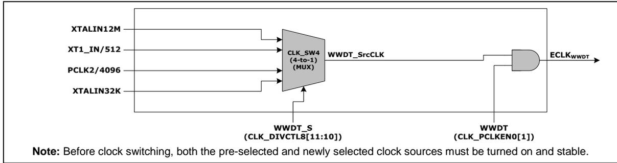
Figure 6.3-13 Windowed Watchdog Timer Clock Divider Block Diagram
