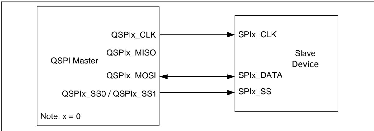
Figure 6.18-10 QSPI Half-Duplex Master Mode Application Block Diagram
