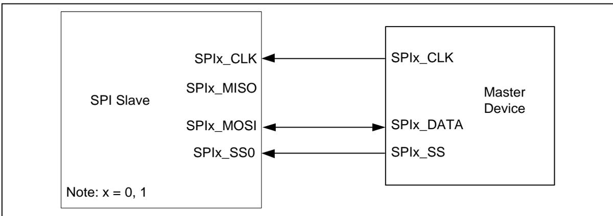
Figure 6.17-11 SPI Half-Duplex Slave Mode Application Block Diagram
