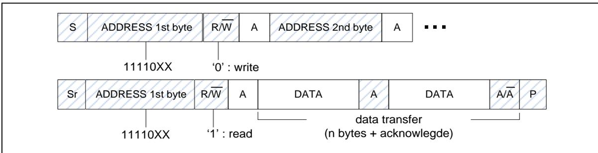
Figure 6.16-10 Master Reads Data from Slave by 10-bit
