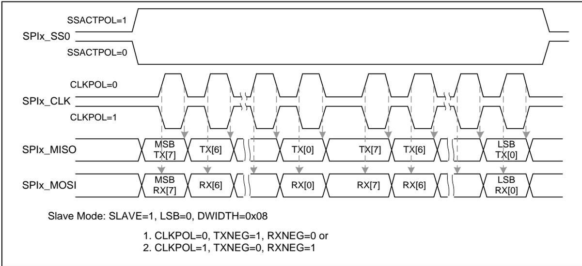
Figure 6.17-19 SPI Timing in Slave Mode
