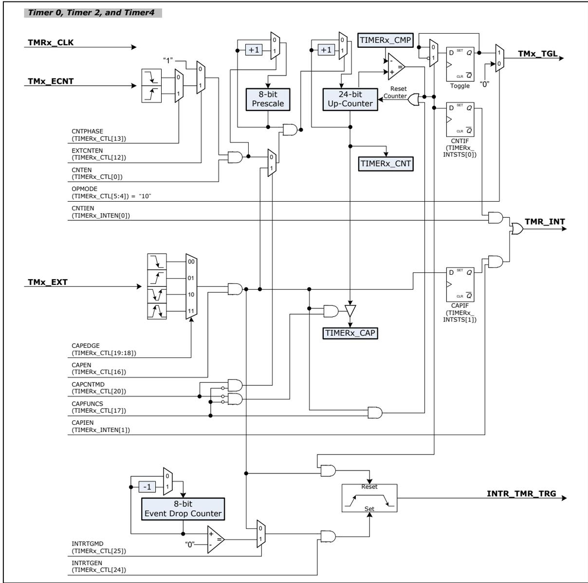
Figure 6.9-1 Timer 0, Timer 2, and Timer 4 Controller Block Diagram
