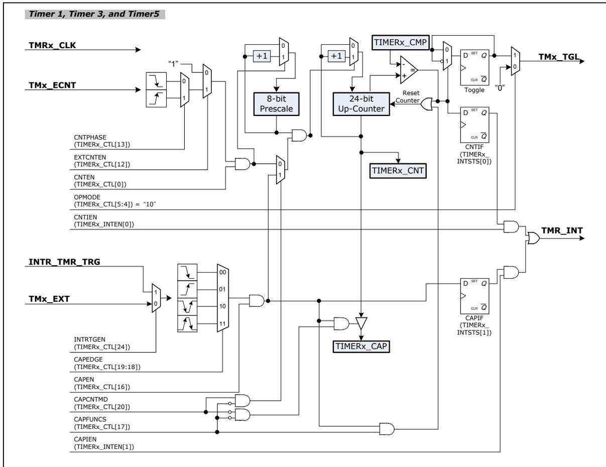
Figure 6.9-2 Timer 1, Timer 3, and Timer 5 Controller Block Diagram
